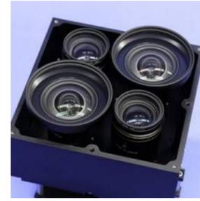
We have substantially upgraded WNISAT-1R mission cameras compared to those on WNISAT-1. WNISAT-1's optical camera had a single sensor capable of observing red, green and blue colors, just like a common camera in everyday use. WNISAT-1R, on the other hand, has four separate cameras dedicated to four separate wavelength bands, leading to a greater resolution and wavelength selectivity.
