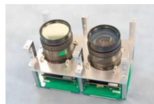
WNISAT-1 is equipped with optical cameras to monitor sea ice. The required ground resolution was as low as 500m, and we pursued very low cost by composing them of lens modules and image sensors built for terrestrial applications. We confirmed the tolerance against space environment through various environmental tests. The camera for near-infrared band will be used to distinguish clouds from ice, both of which look the same in the visible wavelengths.
