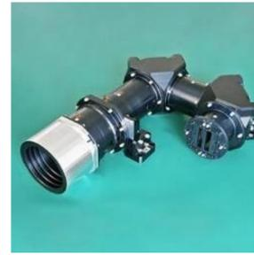
Hodoyoshi-1 carries an optical system capable of obtaining images with the ground resolution of 6.7 m. It uses CCD sensors in the blue, green, red and near-infrared spectral bands respectively. Near-infrared data will enable us to study the growth and health state of plants, which is undetectable with the visible bands alone.
